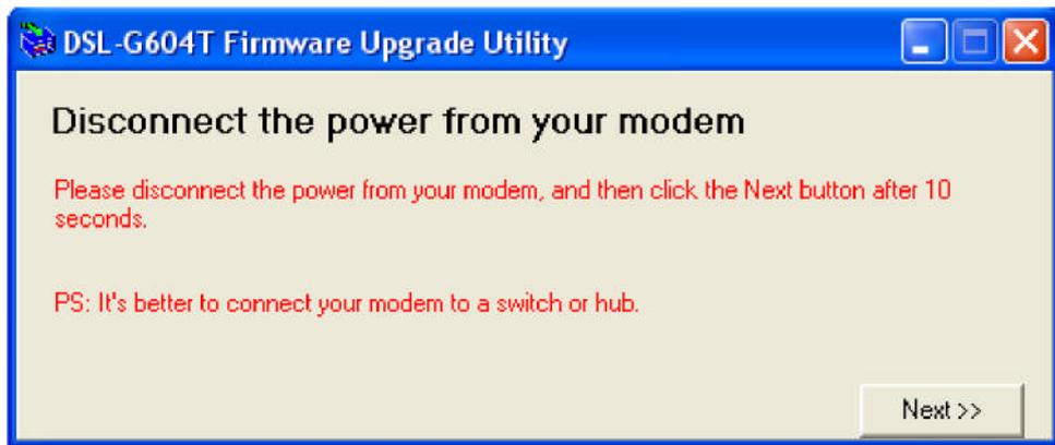
Disconnect the “Power” of the modem/router ADSL, then click on “Next” after 10 seconds.
